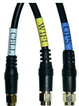
SMA male fitted with identification bands
