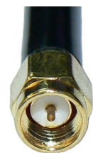
SMA male termination as base of whip
